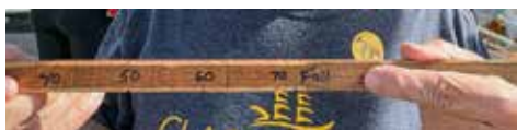
John Lebens with 5-foot long dipstick containing labelled lines to read fuel level. photos by K Weber
