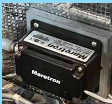
Installed Maretron flow sensor. photo K Weber
