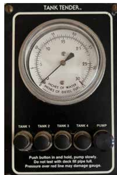
Compadre’s fuel measuring device. The plunger pump is on the far right. The Tank Tender came with the boat. Note: it is all analog. photo provided by K Weber
