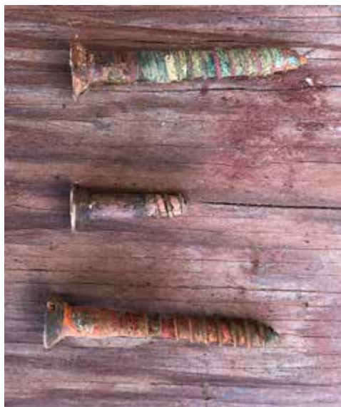
Bronze fasteners removed from the transom showing different states of erosion. Photo courtesy of T Tucker.
