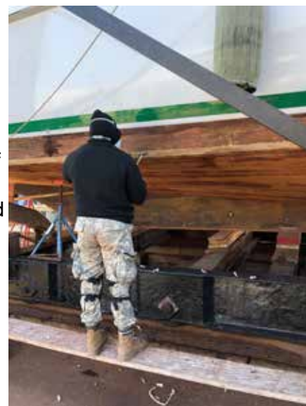
Boatworks crew member with mask removing paint. The bare mahogany planks are visible as are the keel and worm board. Photo courtesy of M Linder.
