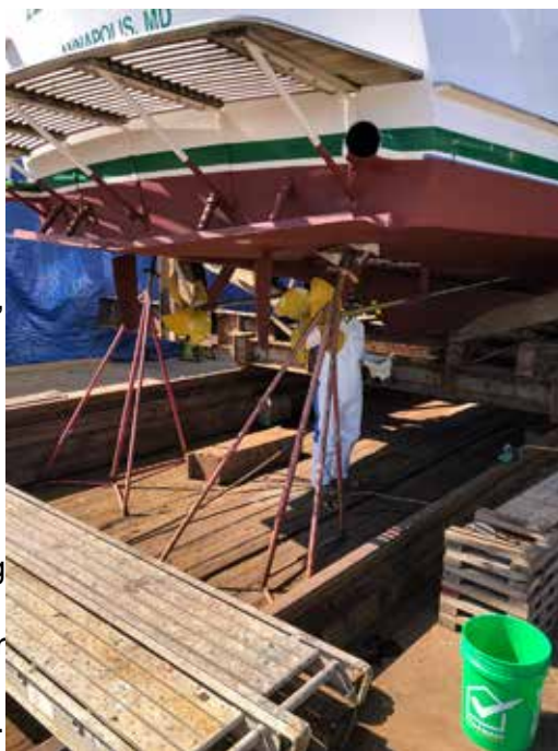
Below waterline all painted and Prop-speed being applied to props and shaft as final preparation for launch. Photo courtesy of M Linder.
