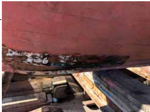
Flaking paint near the bow stem at the worm wood and keel. Photo courtesy of M Linder.
