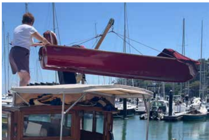
Using the davit to launch the dinghy. photo courtesy of R Sesar
