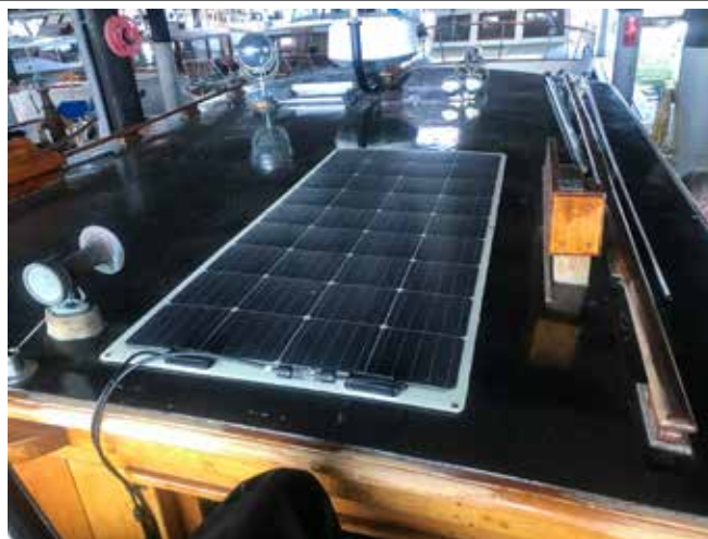
A 175-watt solar panel installed on Larry Benson and Tina Stotz's The Ionius . The panel is 28 inches wide and 60 inches long. photo provided by K Meyer
