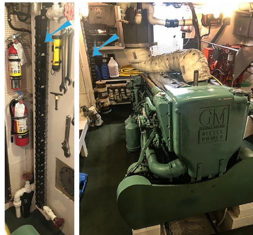
The vertical glass registers/fuel gauges (see blue arrows) were installed before the engine and the upper decks were closed. There are two tanks on either side of the engine room. Each holds 300 gallons. The 1947 engine is still working away.
