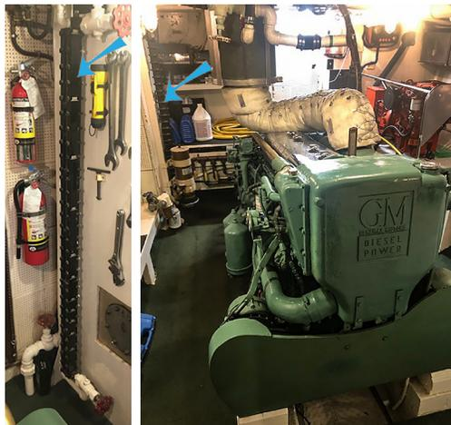
The vertical glass registers/fuel gauges (see blue arrows) were installed before the engine and the upper decks were closed. There are two tanks on either side of the engine room. Each holds 300 gallons. The 1947 engine is still working away.
