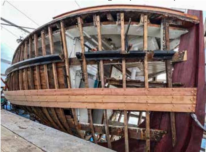
Three planks installed on the starboard side. Note how they fit into the rabbet on the stem. photo by W Shain
