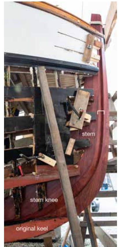
Photo showing rabbit (see bracket) carved into stem and stem knee and continuing down to original keel. photo by W Shain
