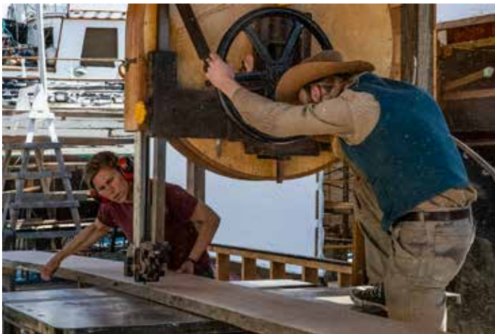
Shipwrights Esther and William cutting the first plank using the ship saw. Esther is feeding the board along the line on the board. William is adjusting the saw to match the bevel indicated at each station. photo by W Shain
