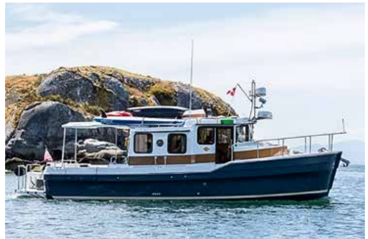
Nordic Tug 31. Length: 35 ft; beam 11 feet, 4 inches photo provided by R Randall & T Powell
