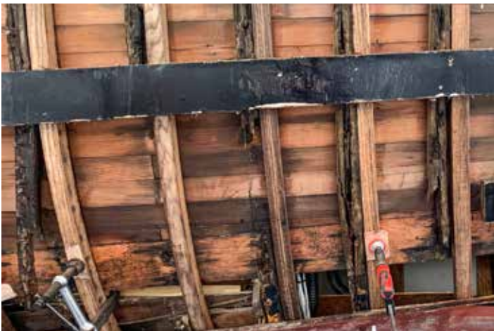
A portion of Comrade 's starboard side with new white oak frames (lighter colored vertical pieces) next to portions of darkly stained old frames. photo by W Shain
