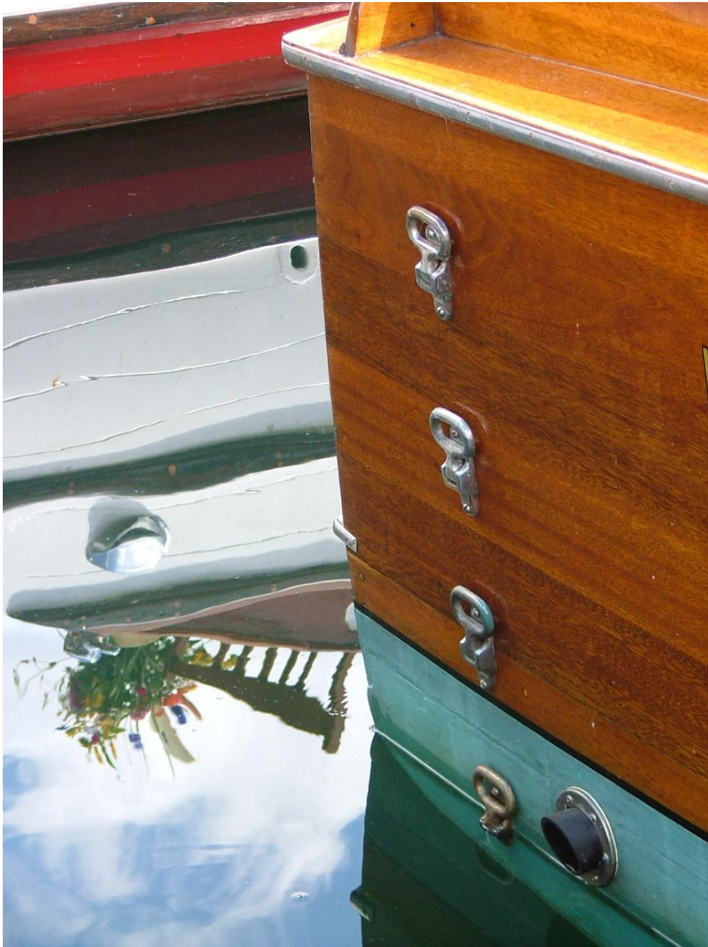
Transom steps on Peaceful , a 1939 26' Richardson, owned by CYA members Tom and Jessica Freeman.
