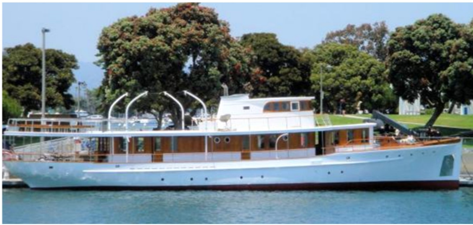
Sobre las Olas . Length: 105' LOA. Beam: 22'. Draft: 8'. Speed: 8-10 knots. Range: 5000 miles. Water: 2,700 gallons. Fuel: 5000 gallons. Range: 5000 miles.
