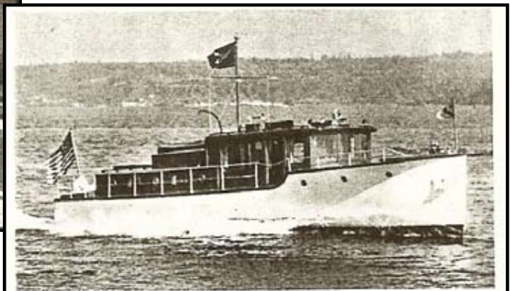
"Pamabro", Owned by Frank Anderline of Seattle She is a 45-footer build by W. J. Schertzter of Seattle. A Hall-Scott Invader engine drives her 20 m.p.m.
