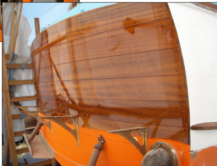
▲ The transom was rebuilt, a dozen or so planks were replaced, the knee of the stem was replaced.
