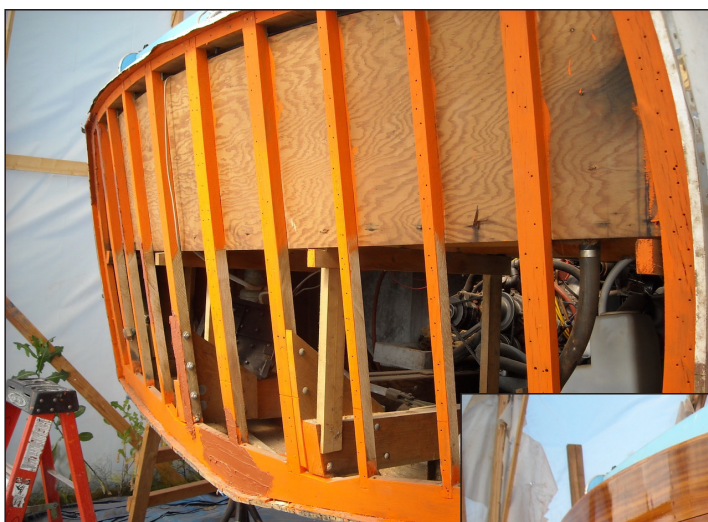
▲ The transom was rebuilt, a dozen or so planks were replaced, the knee of the stem was replaced.
