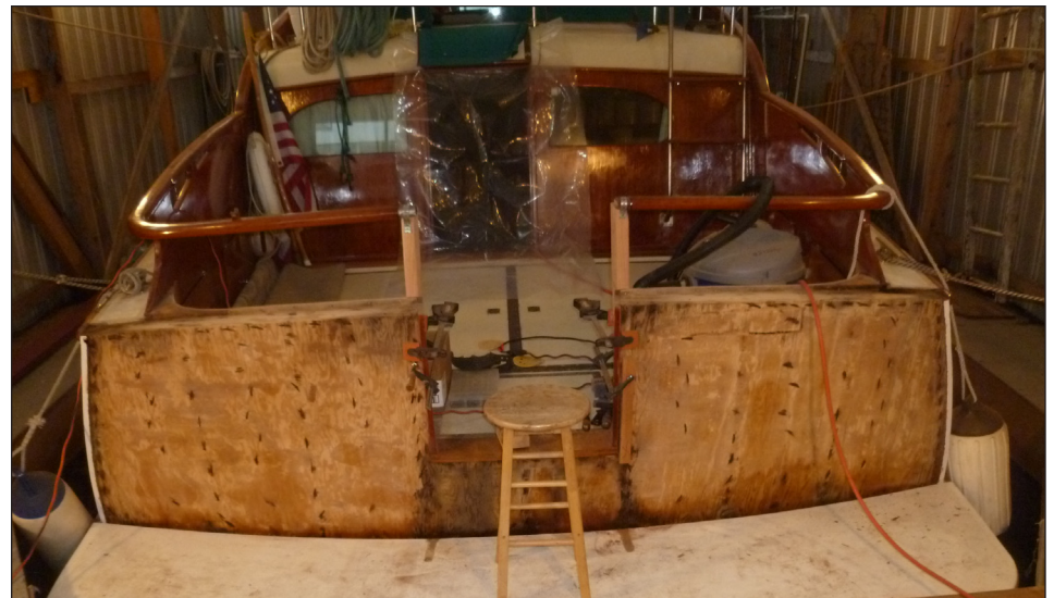
▲ The decorative fairing boards were made of steam bent oak and provided a vertical trim surface on the inside of the cockpit and adjoining the covering boards.
