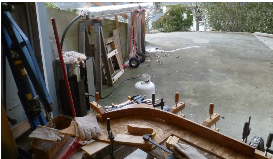
▲ I had some Meranti (Red Philippine Mahogany) that would look good so we milled a piece, 1/2 inch thick and put it in the steamer.
