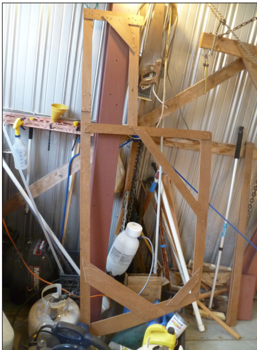
Batten patterns were made for each side (see picture #4), laid on the plywood, marked out and then cut out and installed.
