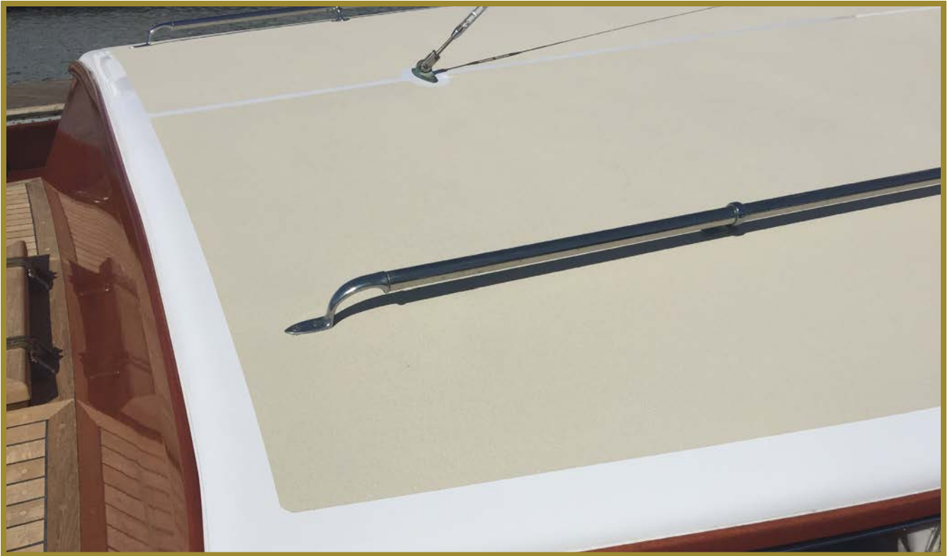
A beautiful moondust non-skid pattern was laid out on both cabin top and fly bridge.
