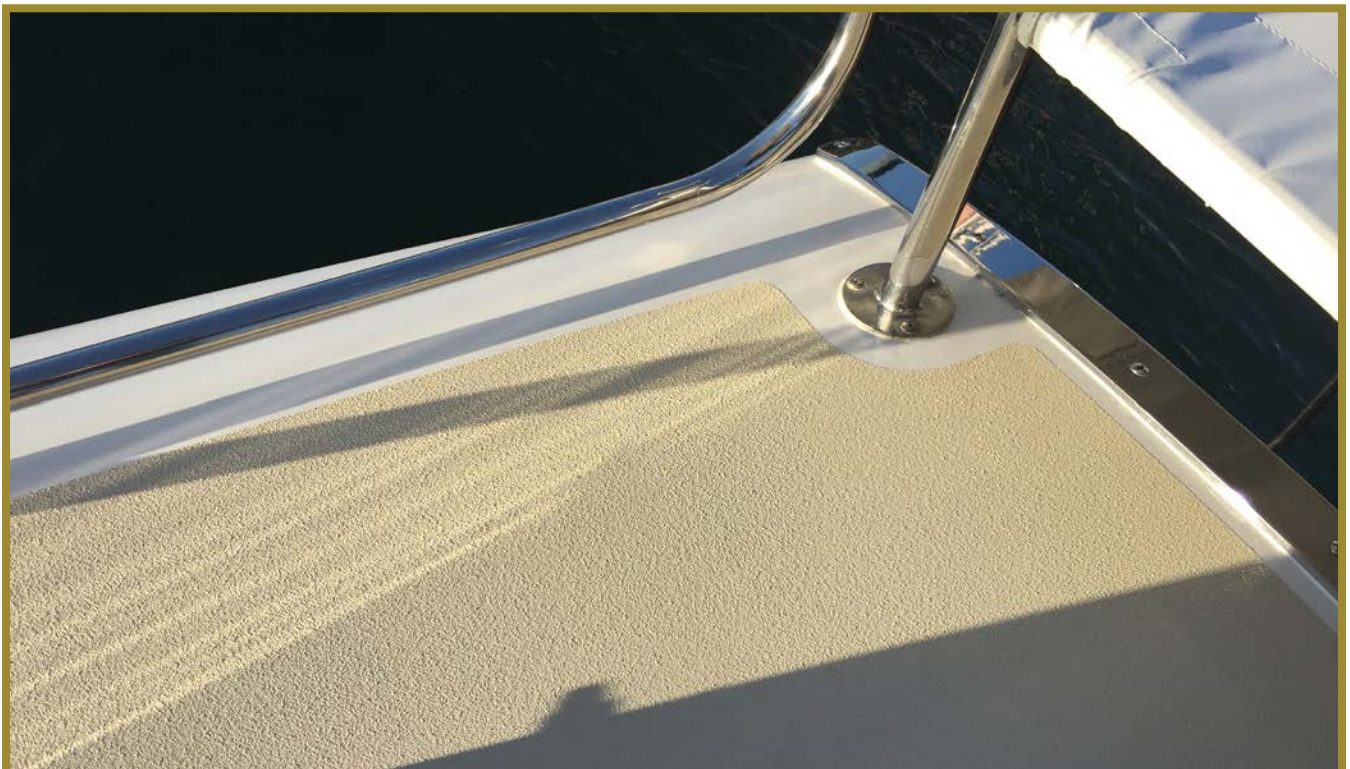
A beautiful moondust non-skid pattern was laid out on both cabin top and fly bridge.
