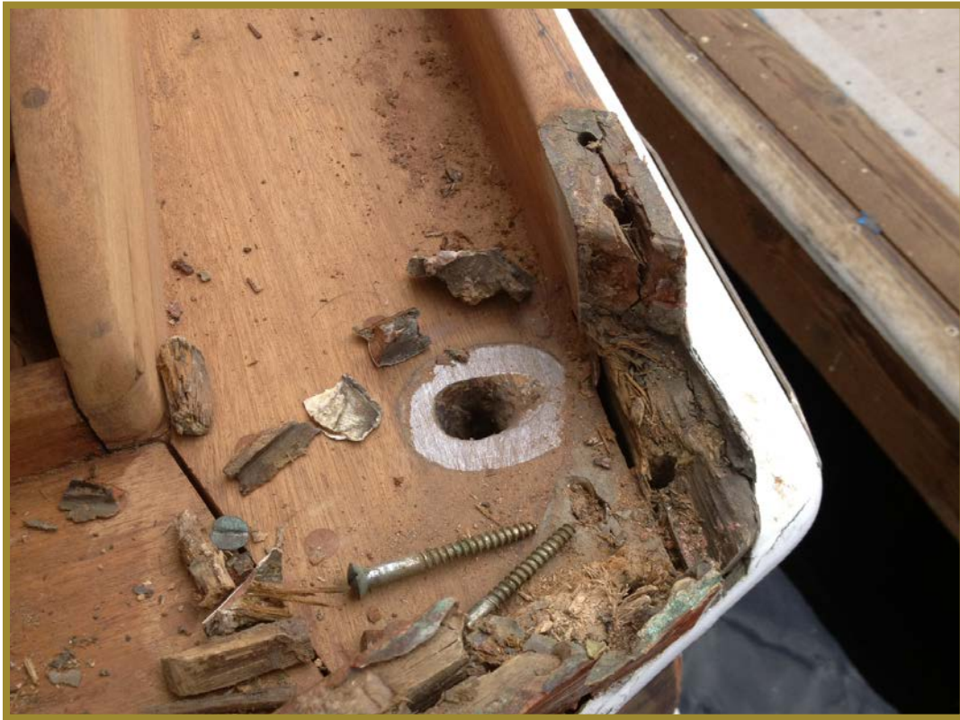
Rotted wood was cut out and inlaid with new mahogany
