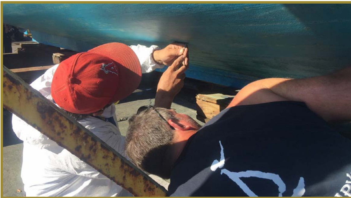
Tony and Pepe, reinforcing the Vera Lee II's hull with over 500 screws to make it perfect.
