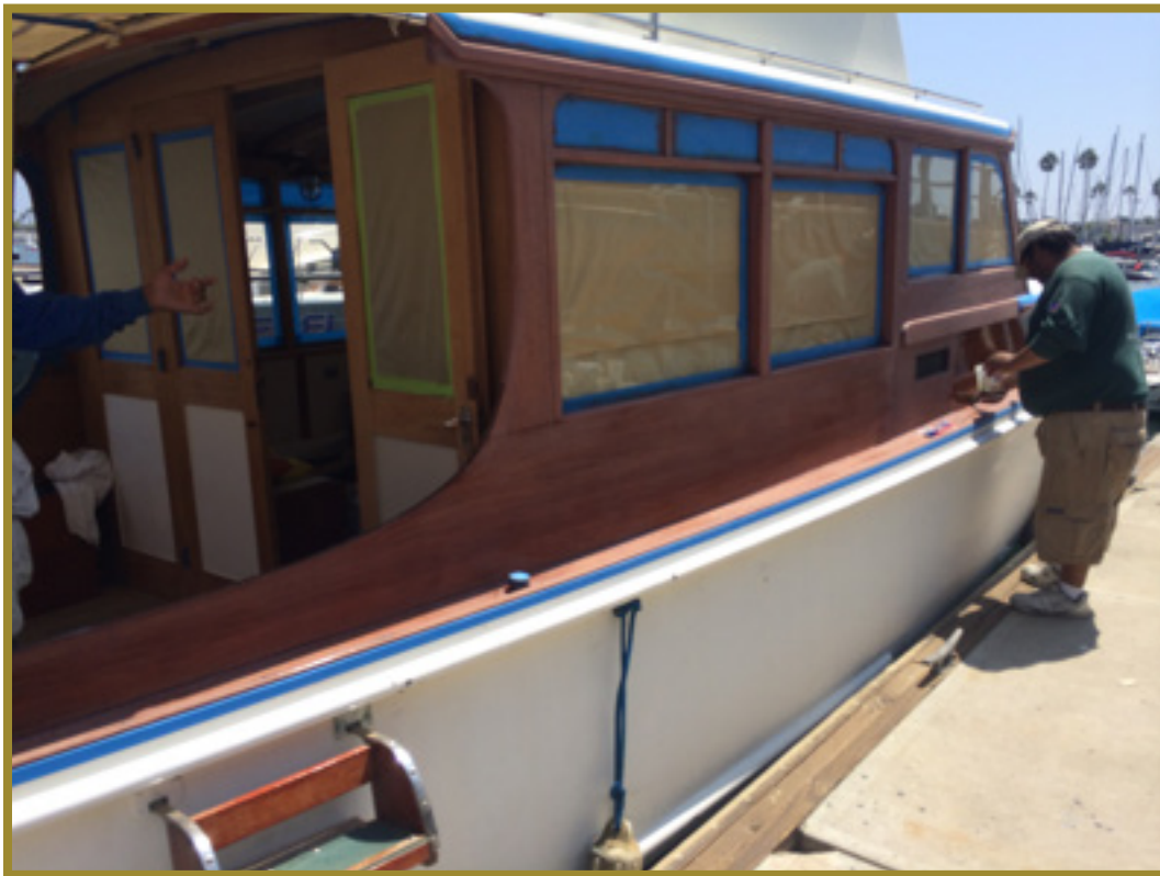
We took on the job of completely refinishing Vera Lee II with a beautiful custom mix of Z-Spar stain and over 12 coats of Crystal by Detco varnish.
