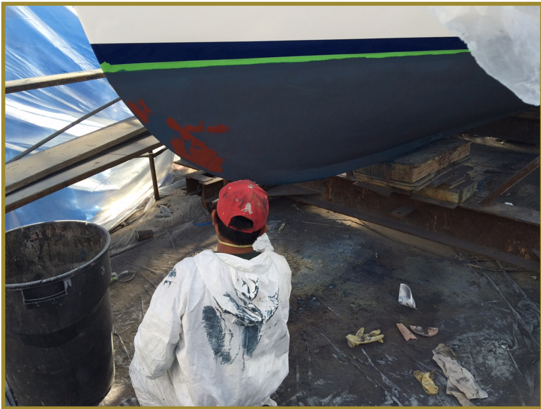
3 coats of Z-Spar pro blue paint were applied to the hull. The first one was mixed with 50% thinner to allow the paint the penetrate the wood easily.
