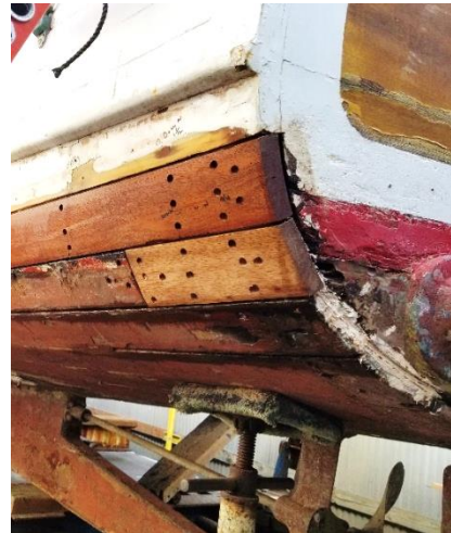
Plank repairs @ port stern
