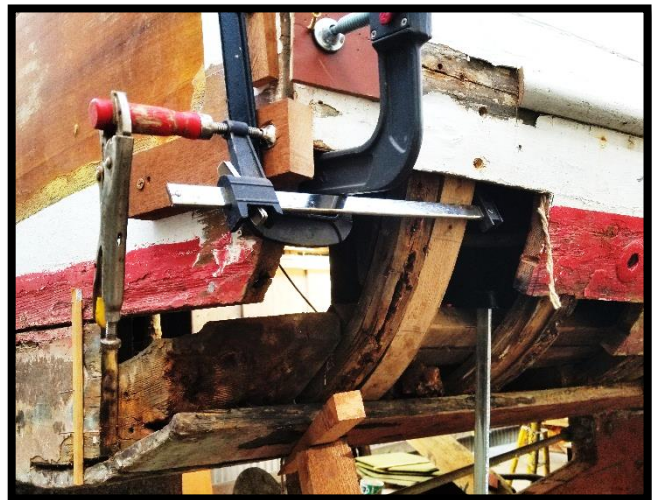
Very compromised ribs are being sistered @ the starboard stern
